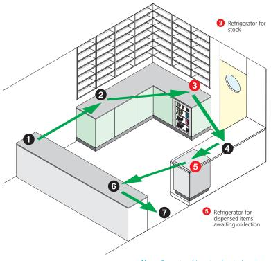
**Above** Separate refrigerators for stock and medicines awaiting collection keep the process of assembly and collection apart, reducing the possibility of error.
